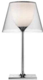
Table luminaire providing diffused lighting. Base, rod support and diffuser support in die-cast, polished Zamak alloy. Polished aluminum tubular. Injection-molded, matte black PA (Nylon) base cover. Injection-molded PC (polycarbonate) opal inner diffuser. Outer diffuser in transparent or fumée PMMA (polymethylmethacrylate).
